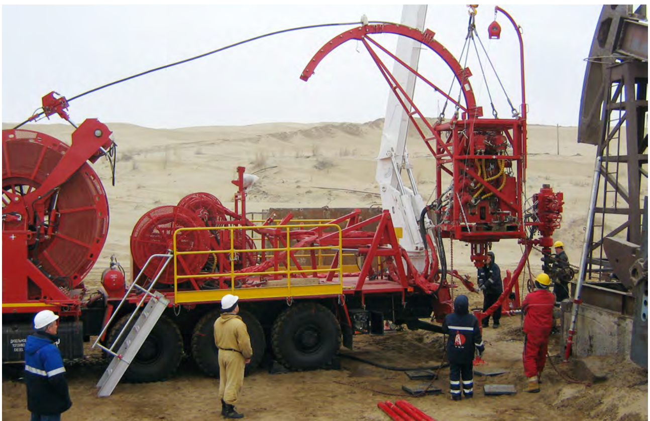
Keymir oilfield: Well acidizing by applying MK30T coiled tubing unit
