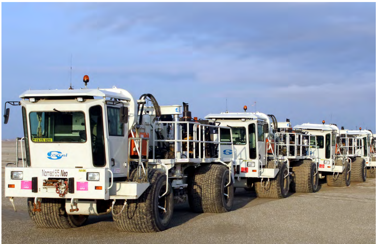
Producing of seismic signal by applying updated Nomad 65 NEO vibro-seis sources (manufactured by Sercel (France))
