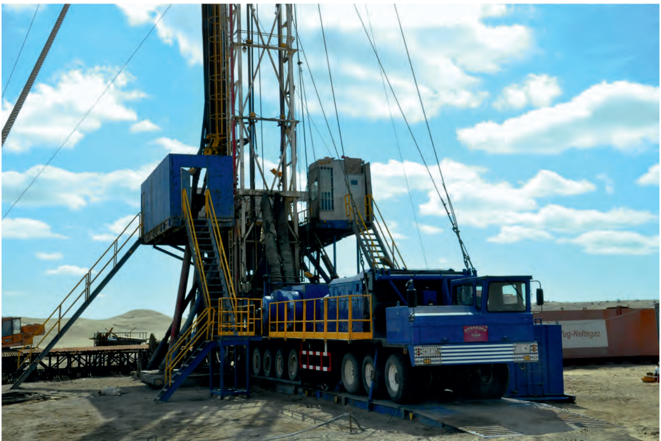
Goturdepe oilfield: Side-tracking by using 225-ton pulling capacity drill rig
