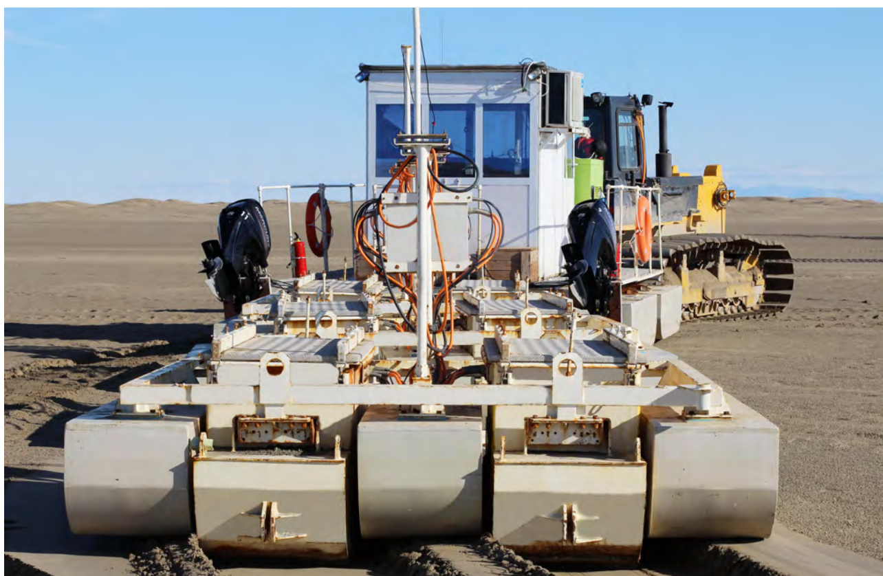
Darja area: Seismic shooting in transition zone by applying pulsed seismic source on a floater towed by dozer (for peat-land operation)
