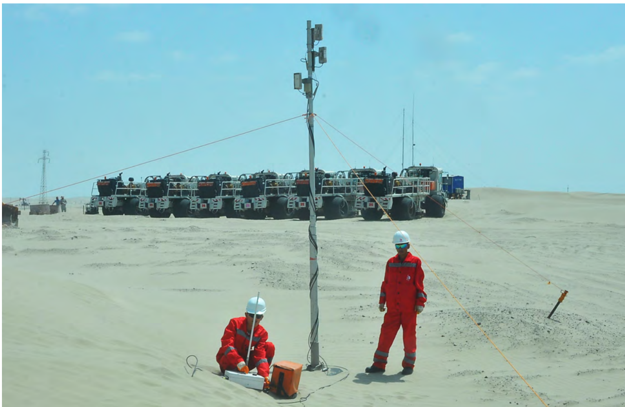
Barsagelmez oilfield: Testing and tuning of Radio-Link transmitter-receiver system of RTS2 wireless seismic data acquisition system (manufactured by Wireless Seismic (USA))
