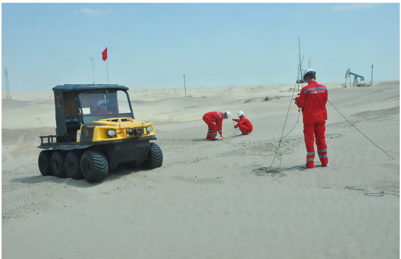
Barsagelmez oilfield: Planting WRUs of RTS2 wireless seismic data acquisition system (manufactured by Wireless Seismic (USA))
