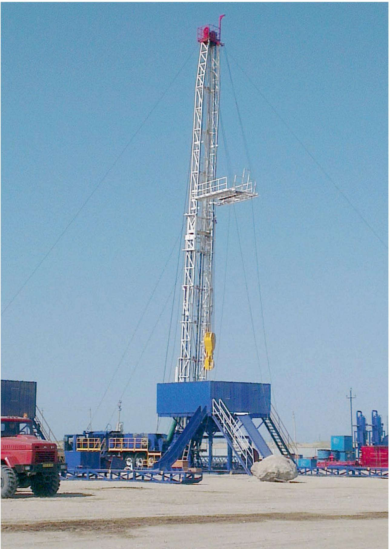
Barsagelmez oilfield: Well work-over in abnormal well operating conditions by using 225-ton pulling capacity work-over rig
