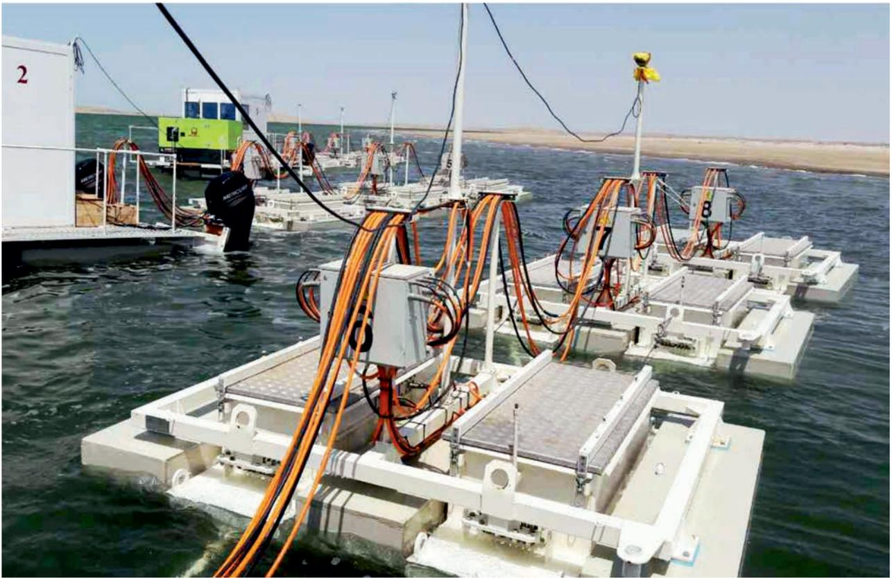
Operation of pulsed seismic source on a floater driven by outboard motors while shooting in shallow waters (to 3m depth)
