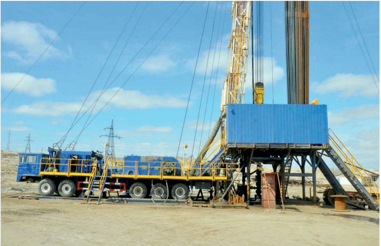
Goturdepe oilfield: Well work-over in abnormal well operating conditions by using 125-ton pulling capacity work-over rig
