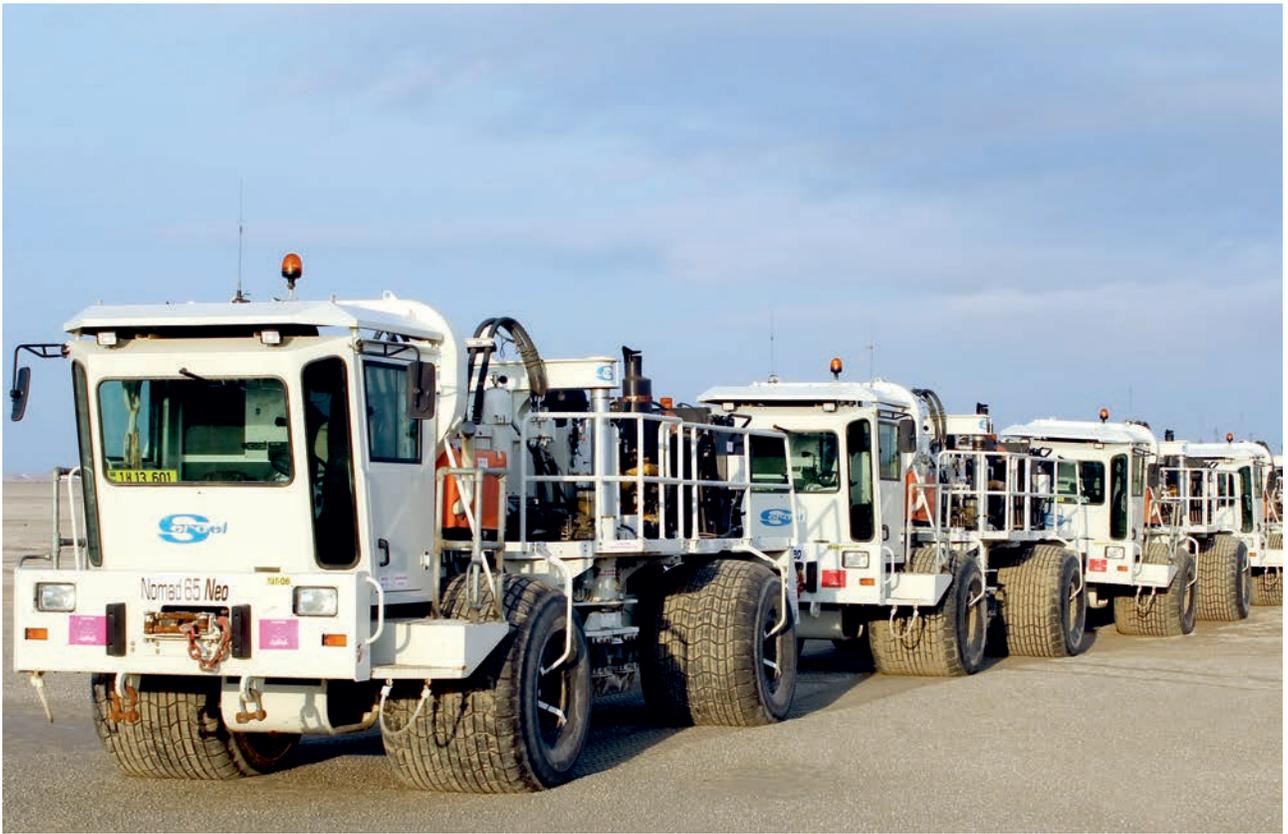
Producing of seismic signal by applying updated Nomad 65 NEO vibro-seis sources
