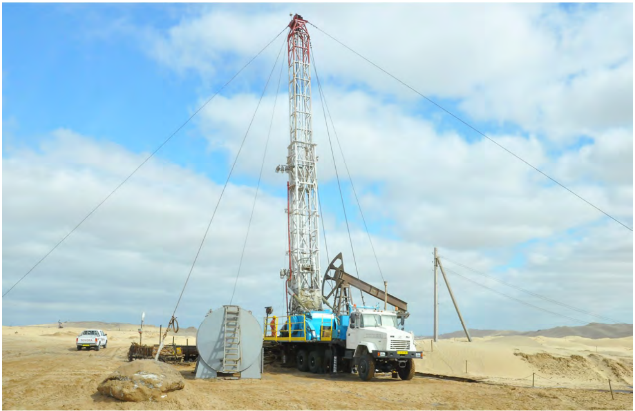
Goturdepe oilfield: Water shut-off jobs by using a workover rig (80 ton load capacity)
