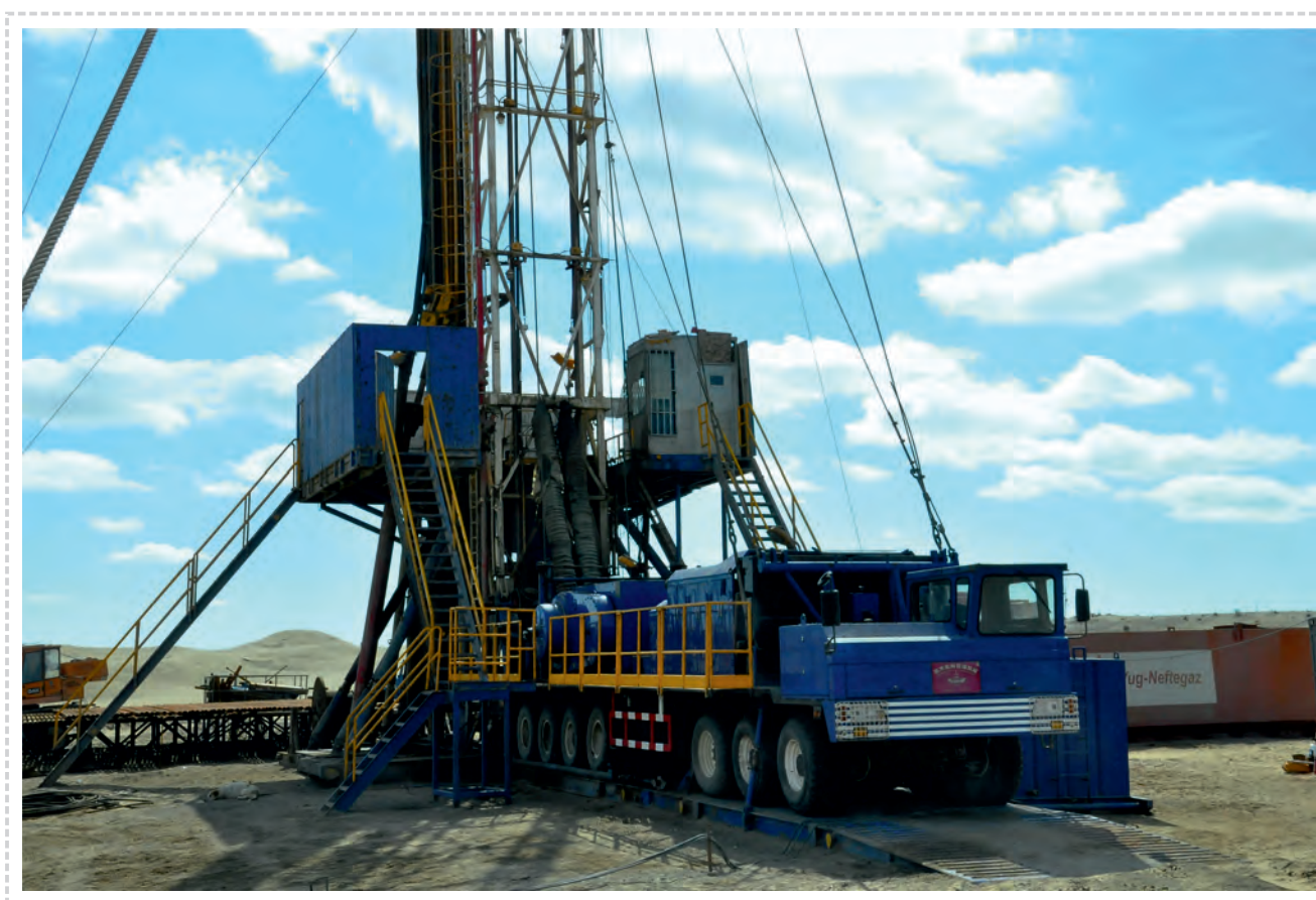
Goturdepe oilfield: Side-tracking by using ZJ-40 mobile drilling rig (225 ton load capacity)
