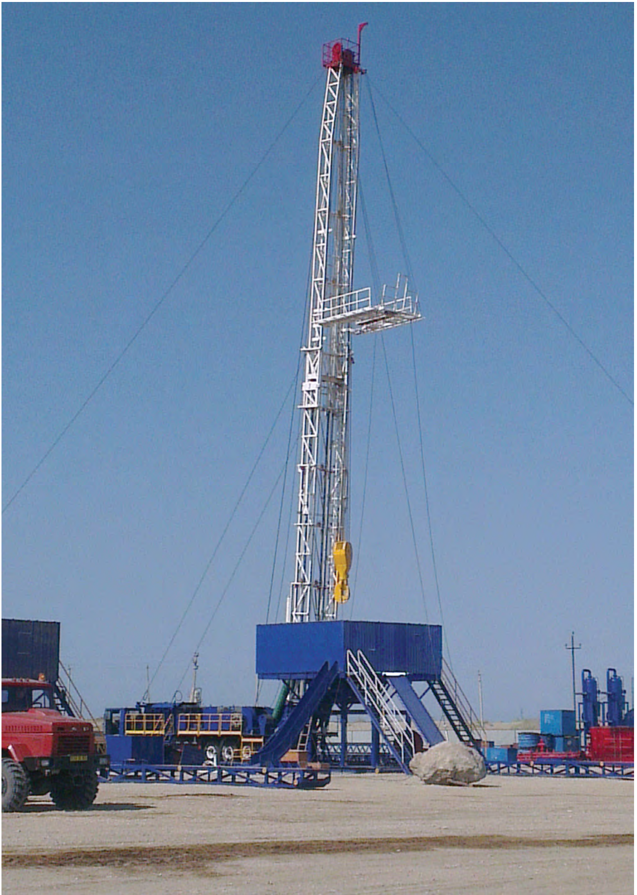
Barsagelmez oilfield: Well workover job in abnormal operating conditions by using ZJ-40 mobile drilling rig (225 ton load capacity)
