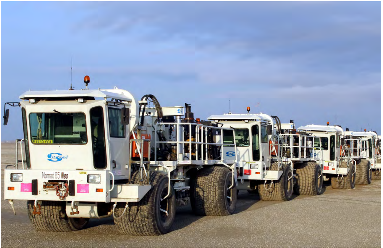
Goturdepe oilfield: Generating seismic signal by applying updated Nomad 65 NEO vibro-seis sources (manufactured by Sercel (France))
