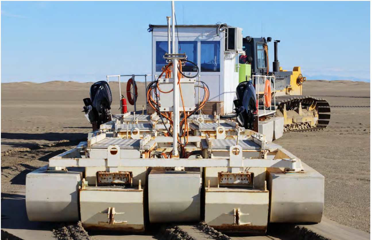
Darja area: Seismic shooting in transition zone by applying pulsed source on a floater towed by dozer (for peat-land operation)
