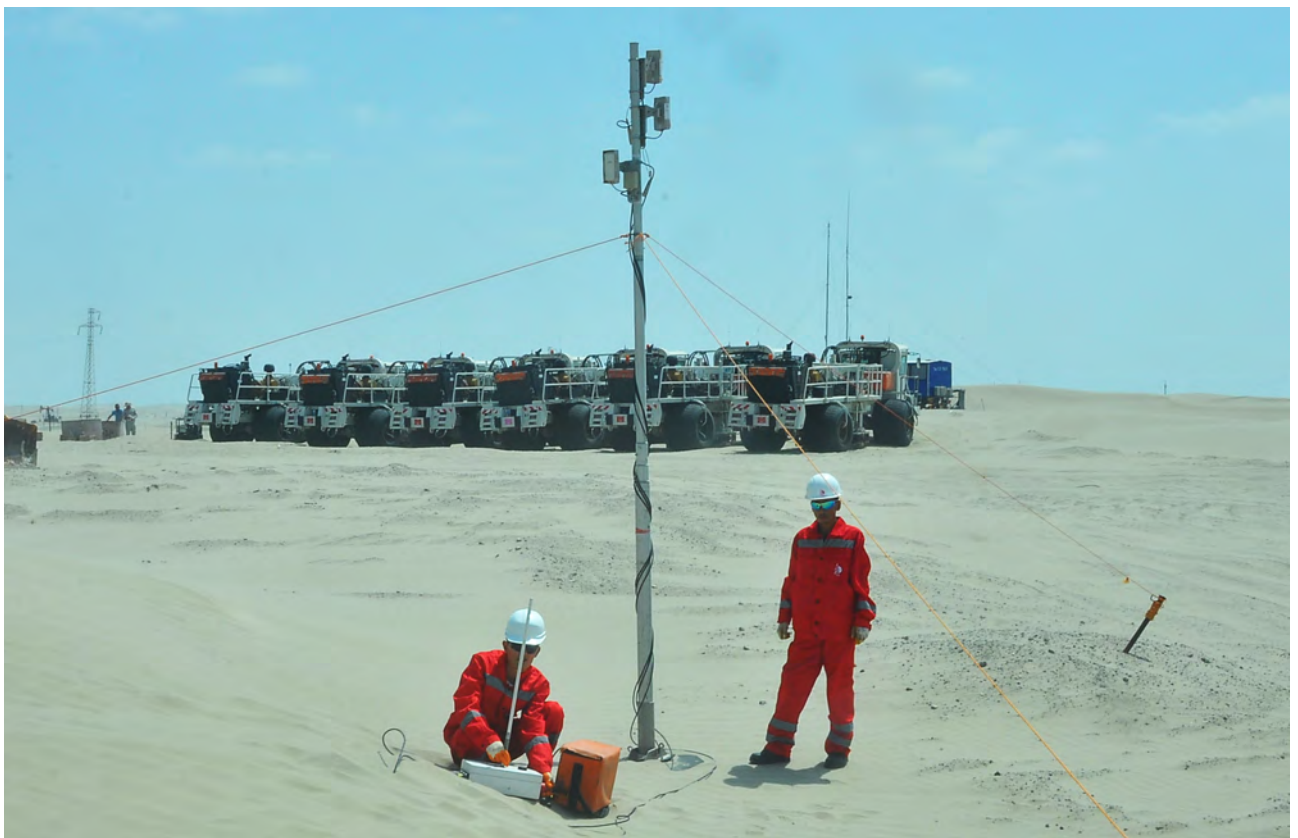
Barsagelmez oilfield: Testing and tuning of RTS2 wireless seismic data acquisition system (manufactured by Wireless Seismic (USA))
