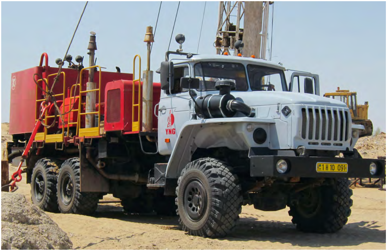
Barsagelmez oilfield: Pumper operation while water shut-off jobs
