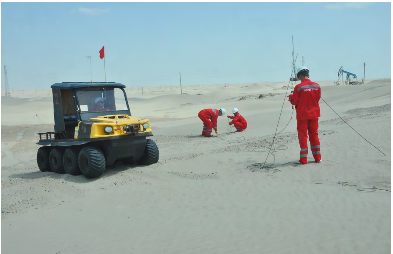
Barsagelmez oilfield: Placing WRUs of RTS2 wireless seismic data acquisition system (manufactured by Wireless Seismic (USA))
