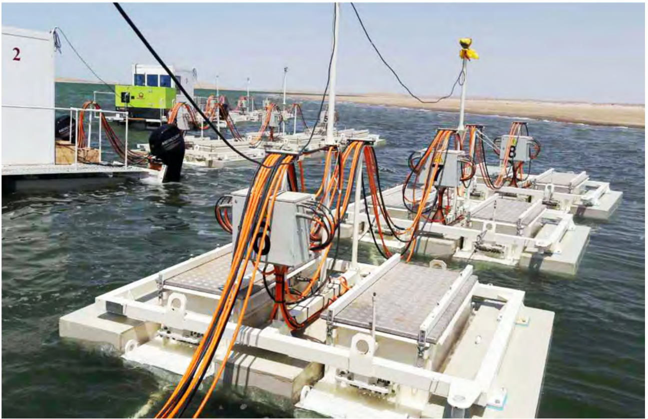
Operation of pulsed source on a floater driven by outboard motors while shooting in shallow waters (to 3m depth)
